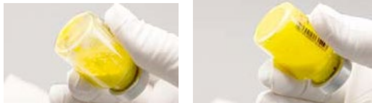
Unsuspended: visible clumps Suspended: no clumps Figure B: Check for unsuspended powder and repeat tapping if needed.
